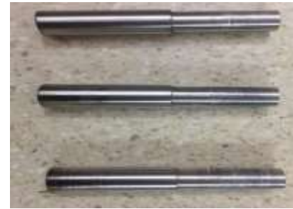
Fig. 4. Different FSHE tools used for hole expansion
